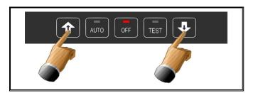
Step 6: Press the "OFF" button to move to the next phase or until the word "End" appears on the screen. To exit hold the "OFF" button at any time for 4 sec.
