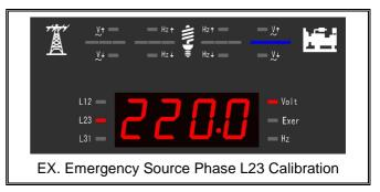
Step 4: Use a good quality voltmeter as a reference to calibrate the ATS-385 voltage reading to the desired phase.
